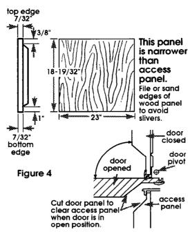
Heavy-duty door springs must be used if custom door panel weighs more than 4 pounds. Heavy-duty Door Springs Kit, Part No. 4318050, is available from your dealer or parts supplier. Maximum door weight is 8 pounds.
